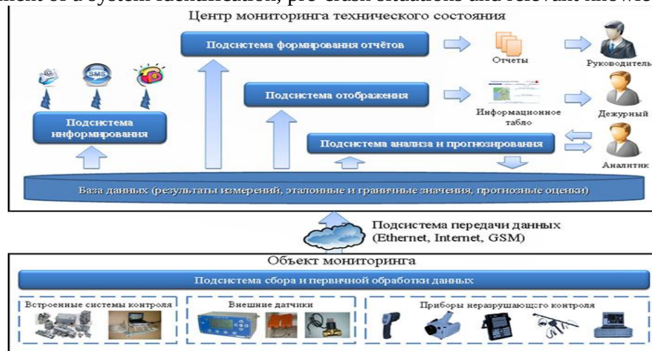
Figure 1 - Architecture of an automated monitoring system
