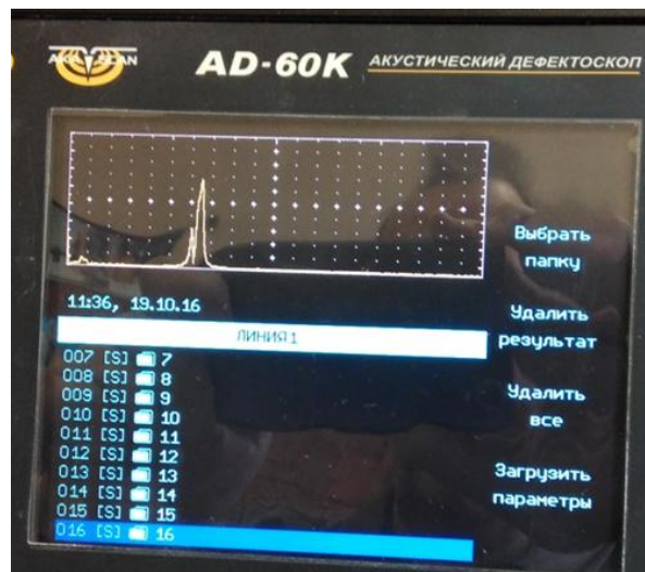
Figure 3 – universal acoustic and impedance defectoscope AD-60K: a –the absence of defects in the structure of CM; b – the presence of defect such as delamination
